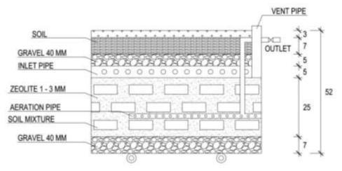
Figure 1. Multi Layer Soil system
