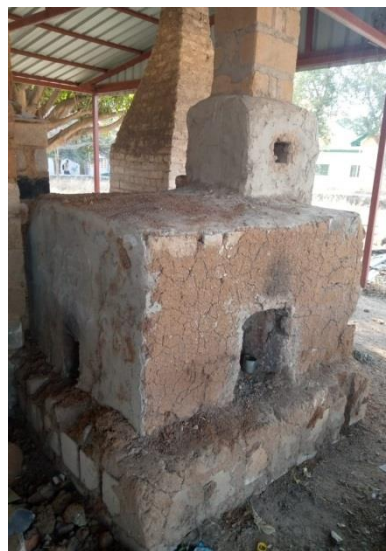
Figure 4. 4.5 Cubic feet (CF) cross draft kiln
