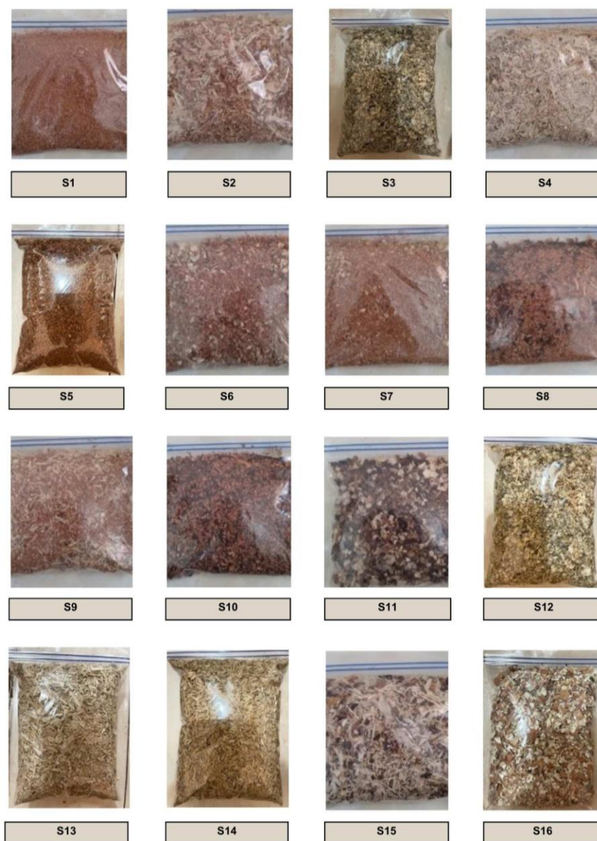
Figure 1. Raw material for RDF production material
