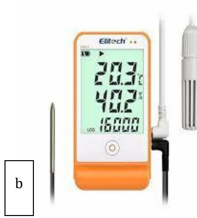
Figure 3. Measurement tools used (a) Dry bulb, (b) Elitech GSP-6
