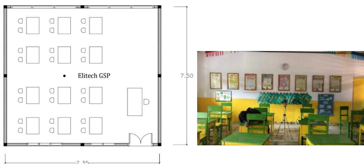
Figure 1. Placement of measuring devices in indoor
